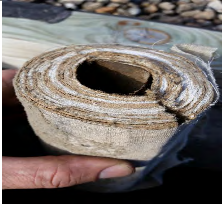
Samples 33-35 Pipe Insulation – Millboard on 1" pipes
